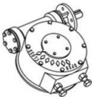
With flange for connecting with actuator, it follows ISO 5210
