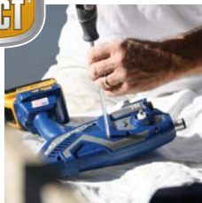
1. Remove the cover with a screwdriver.
